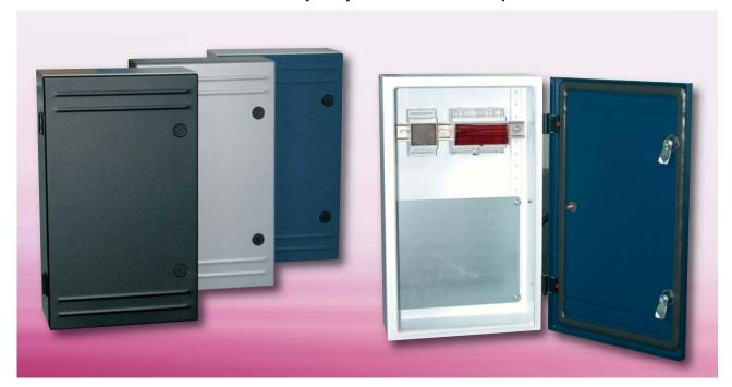
Basic enclosure consisting of wall mounting part with 4 welded fixing brackets and 2 brackets to take the mounting plate and/or mounting rail inside. Front door with foamed sealing, 180° hinges and locking handle.
